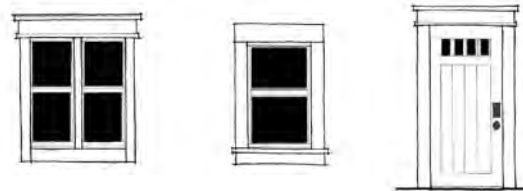
Figure 3.32: The trim accents the vertical nature of the windows and doors. Head and sill trims are tall in nature and side trims are narrow.
