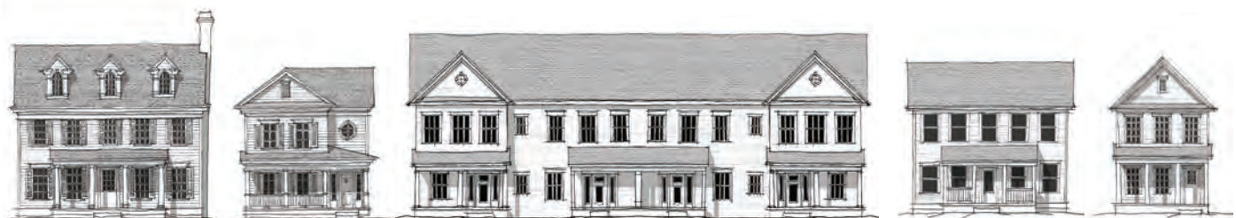
Figure 2.4: A composition of five buildings in varying sizes that employs East Coast styles such as Georgian, Neo-Classical, and Colonial Revival. Simple forms, large gabled roofs that run parallel to the street, and occasional street-facing pediments create a plain yet diverse composition.
