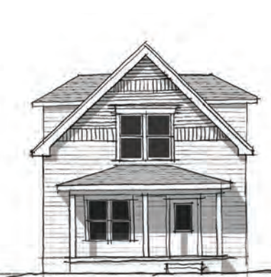
Figure 3.54: The creative design of shingle patterns highlights a gable end.
