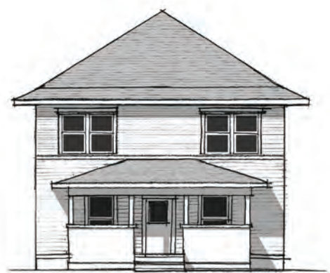
Figure 3.56: Narrow horizontal siding transitions to a wider horizontal siding below, a texture change that emphasizes the building's base and its horizontal appearance.
