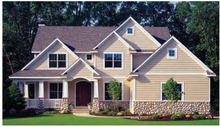
Figures 3.3 and 3.4: A comparison of two buildings that emphasize the importance of creating a legible hierarchy of primary, secondary, and tertiary forms in designing a well-articulated façade. The example on the left (PP) has a simple forward-facing gable (the primary form) with a porch (the secondary form) added and a balcony subtracted on the second floor. The example on the right (PP), on the other hand, employs five forward-facing gables that are competing, making the whole composition too crowded.
