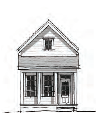
Figure 2.126: A narrow single-story Shotgun building with a steep gable roof perpendicular to the street.
