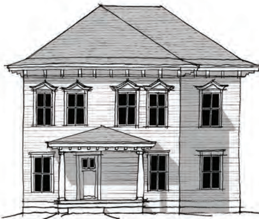
Figure 2.76: A hip roof with skirts, ornate eave brackets, and simple boxy building massing are common features of Italianate style.
