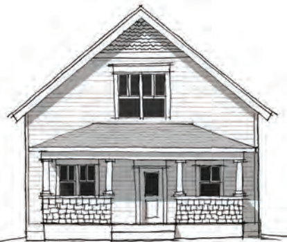
Figure 2.42: A one-and-a-half-story Folk-Victorian house with a full porch. Half-stories are common in this style.
