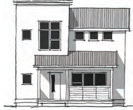
Figure 2.60: Occasional flat roofs with modern-style window composition may add interest to the mix on a block face.
