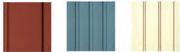
Figure 3.60 (PP): Various vertical siding examples include (left to right) vertical panels, board and batten, and beaded soffit.
