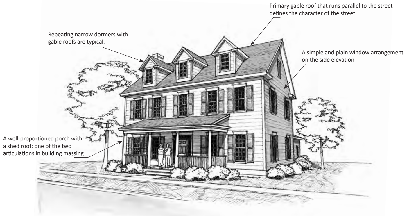
Figure 2.91: A prototypical building in a simplified Georgian style, which is common in the East Coast.
