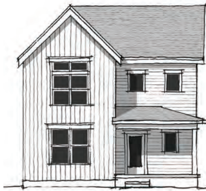
Figure 3.55: Board and batten on a tower element emphasizes verticality.
