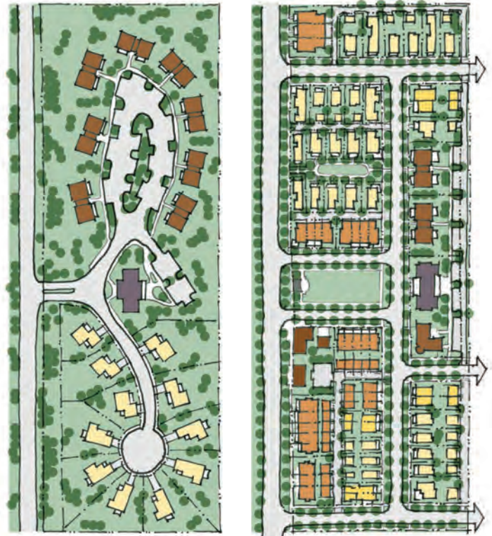
Figure 1.7: A comparison of a conventional suburban pattern (left) with a street-oriented traditional neighborhood site design (right). The conventional plan has a single entrance with branching access roads where parking is provided at the front of homes (either as surface parking or attached garages) and where buildings are located away from the roads. The traditional neighborhood plan provides multiple access points via a street grid, and the civic buildings are highlighted by a centrally located neighborhood park. Alleys provide vehicular access and allow sidewalks to serve uninterrupted as pedestrian pathways. Buildings are placed closer to the sidewalks, shaded by street trees located in the tree lawns.
