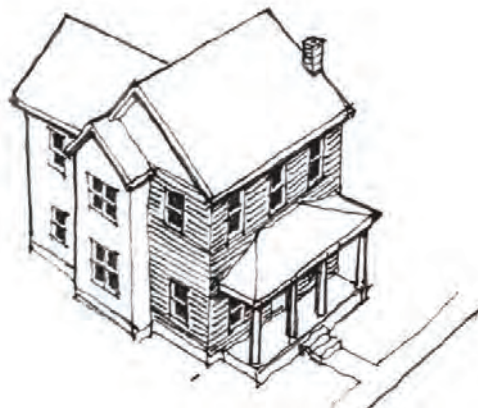
Figure 3.40: Material and color change should occur at interior (concave) corners as opposed to exterior (convex) corners of a building. From The Design Book: The Northern Neighborhoods , Stapleton.
