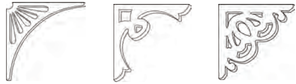
Figure 3.30: Brackets can be both structural and ornamental. Scrollwork adds interest to a building's character.
