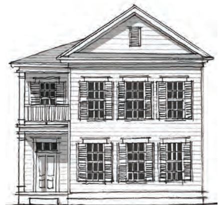
Figure 2.128: A two-story side-porch building with a low-sloped gable and a classical pediment facing the street.
