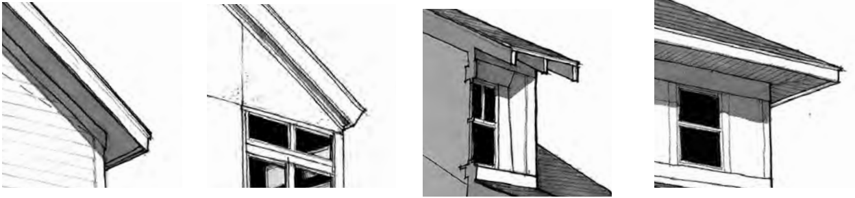
Figure 3.11: Variations that contribute to defining a building's architectural style include (left to right) enclosed soffits with plumb-cut eaves, minimal overhangs with square-cut eaves, exposed rafters, and soffit materials.
