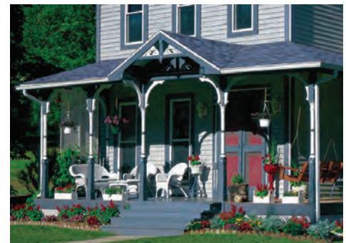
Figures 3.22, 3.23 (PP), and 3.24 (PP): Three examples of amply-sized porches that express the character of their architectural styles. The primary elements to consider are column sizes, bases, and capitals.
