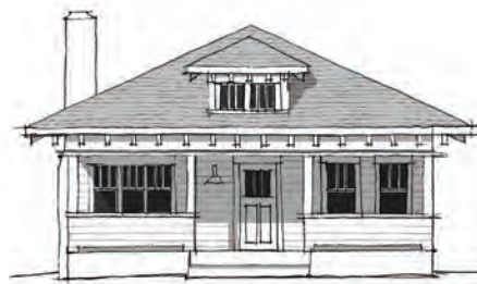
Figure 2.16: A single-story example with a hip roof. Note that the porch roof is an integral part of the primary roof form.
