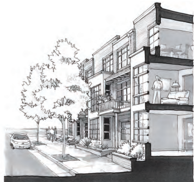
Figure 1.8: Section-perspective drawing of a three-story apartment building placed close to the sidewalk, creating an urban character that may be proper for certain parts of the neighborhood. From The Design Book: The Northern Neighborhoods , Stapleton.
