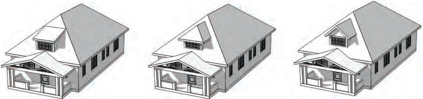
Figure 3.9: Three of the most common dormer types are illustrated on the building above: from left to right, a shed roof dormer, hipped roof dormer, and a forward-facing gable dormer. Note that the dormers in all examples qualify as articulations that increase interest and make the buildings more friendly.
