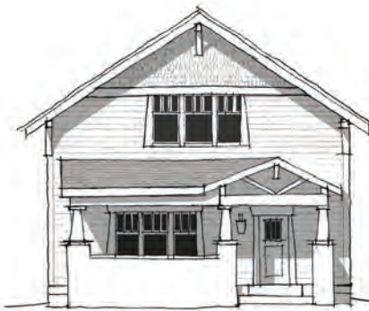
Figure 2.25: A two-story example with a unique porch articulation. Note the low plate height of the second floor.
