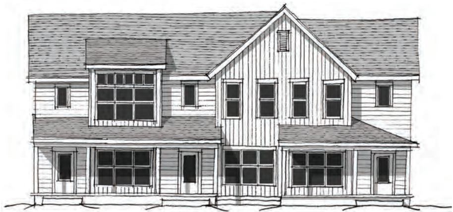
Figure 2.51: A three-unit townhouse building with articulation that reduces the intensity of the building mass, avoids repetition, and unifies the façade. Note the setbacks on the second floor and the simple rectangular footprint of the building.
