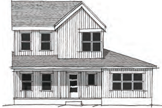
Figure 2.59: A single-story part of the building integrated to the two-story section via the roof form. This example is a more modern interpretation of the style.
