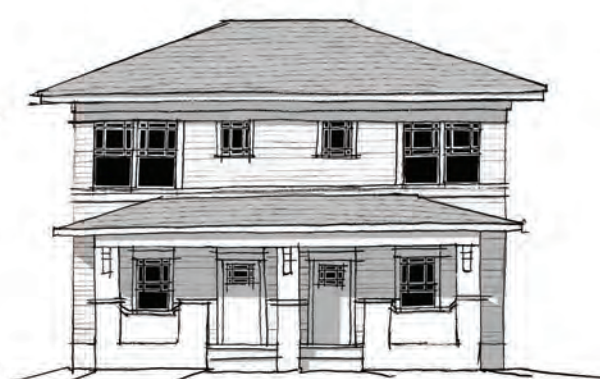
Figure 2.68: A duplex building with symmetrical façade arrangement. The continuous bands, window and door types, and column ornaments are typical of Prairie style.
