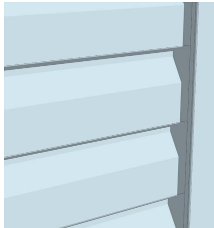
Figure 88 (i-88a, i-88b): At the receiving pocket, vinyl siding may create an unwanted shadow line. With Dutch lap, the shadow line is limited to the upper corner. Other profiles with minor shadow lines include beaded, vertical, flat, insulated clapboard, and some narrow, restoration-style clapboard.
